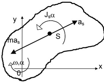
$$\begin{aligned}\sum F_{ix} + m(-\ddot{x}_s) &= 0 \\ \sum F_{iy} + m(-\ddot{y}_s) &= 0 \\ \sum M_s + J_s(-\alpha) &= 0\end{aligned}$$
